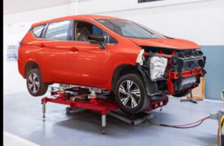
After an accident, the frame of your vehicle may become misaligned. Our advanced frame correction equipment precisely measures and corrects any frame damage, ensuring that your car's structural integrity is restored to factory standards for maximum safety.
