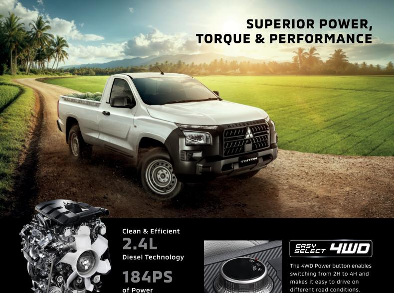
different road conditions. 2H to 4H switching can be done when the vehicle speed is not exceeding 100 km/hr.
